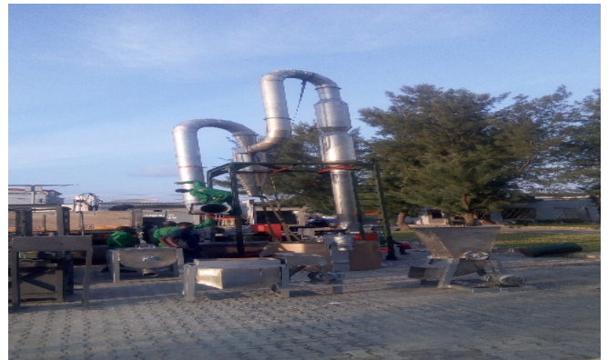
Figure 2: Cassava drying technologies: Solar drying in Uganda (left) flash drying in Nigeria (right)
