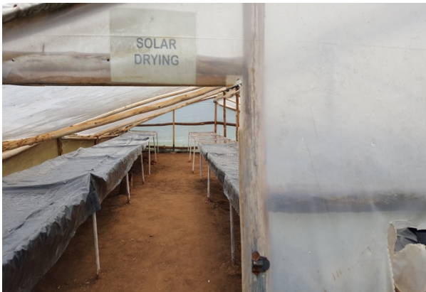
Figure 2: Cassava drying technologies: Solar drying in Uganda (left) flash drying in Nigeria (right)
